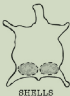
Diagram of a horse hide showing where Cordovan leather is obtained. Sourced from the internet.
